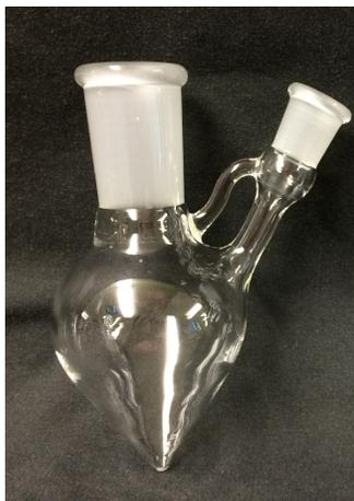
**Figure 7.** Image of pear-shaped evaporation flask with central 24/40 and side 14/20 standard taper ground-glass joint.
